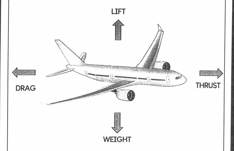
Note that the diagram must include a clear direction, for example the nose of the plane shows the direction the plane is flying. Thrust is always in the direction of motion.
